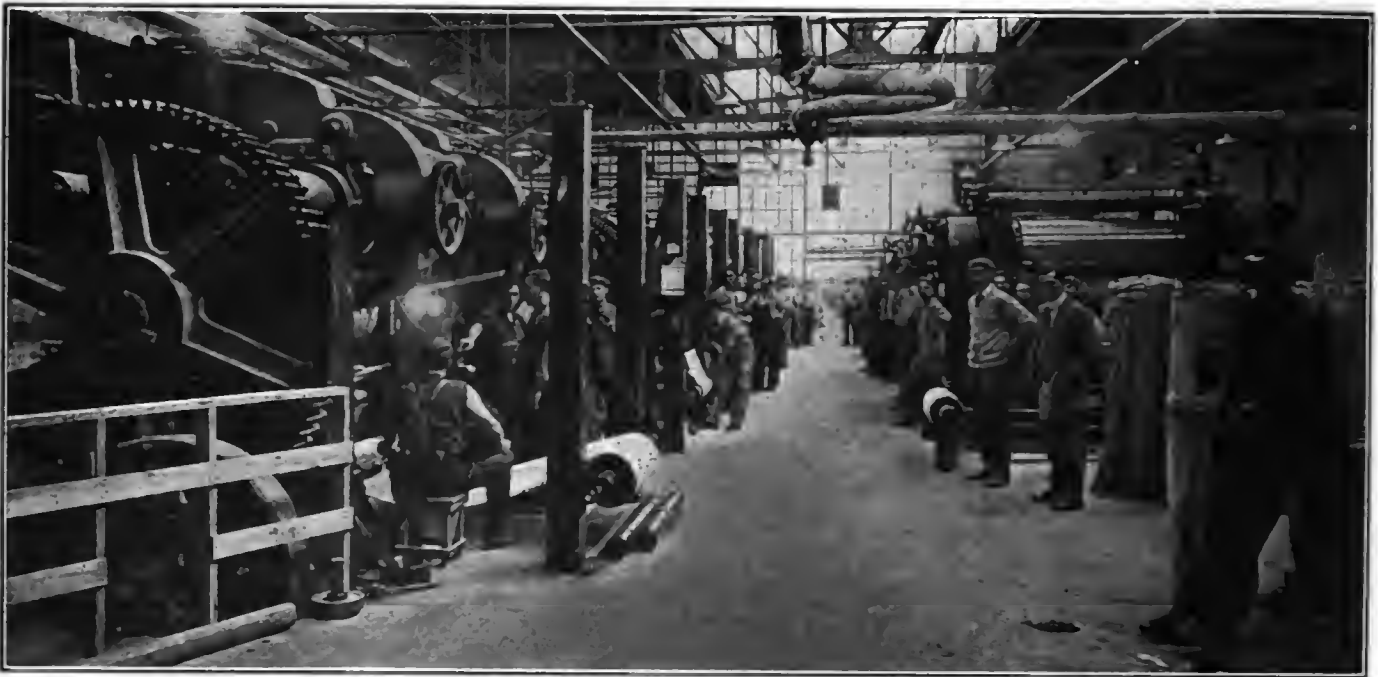
The calender room where the rubber stock is passed through the heated rolls of the huge calenders.
